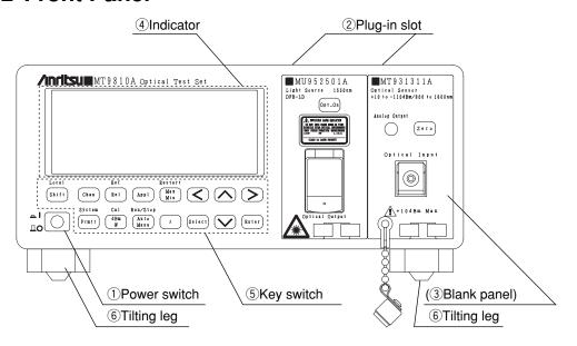
(1) Power switch A switch to turn ON/OFF the power source.
