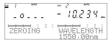
Fig. 4-5 Screen during Execution of Zero Setting
