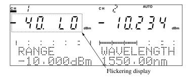
When the minimum range of -90 dBm is set in the AUTO RANGE or MANUAL RANGE mode, if light that falls below -100 dBm is input, the measured value (numerical value) remains displayed and the dBm representation that constitutes the unit flickers to signify the underrange. Moreover, when light that falls below -120 dBm is input, indications of "-130," the value that is the range display minus 40 dB, and "LO" flicker to signify the underrange.
