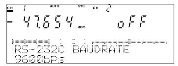
Fig. 4-51 RS-232C Baud Rate Setting Screen
