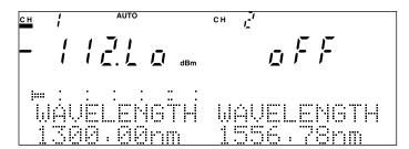
Fig. 4-2 Display upon Completion of Self-Check
