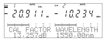
Fig. 4-25 Calibration Measurement Screen
