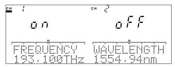
Fig. 4-40 Center Optical Frequency Representation Screen
