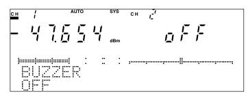
Fig. 4-57 Buzzer OFF Setting Screen
