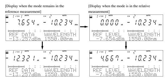
Fig. 4-20 Shift from Reference Measurement to Relative Measurement
