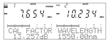
Fig. 4-24 Correction Value (CAL FACTOR) Setting Screen
