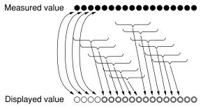
Fig. 4-11 Operations when Averaging Frequency is Set at Five Times
