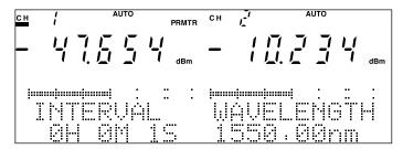
Fig. 4-15 Interval (Optional Value) Setting Screen
