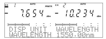
Fig. 4-16 Wavelength Display Setting Screen
