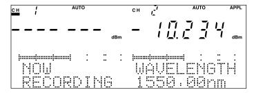
Fig. 4-31 Screen to Set Number of Data to be Recorded (When the Interval is 200 ms or Less)
