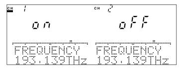
Fig. 4-38 Output Optical Frequency Setting Screen
