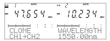
Fig. 4-27 Clone Function Screen
