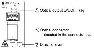
(1) Optical output ON/OFF key Used to switch the optical output ON and OFF.
