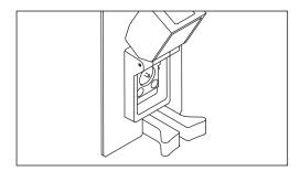
4) Follow the procedures on the other way around to affix the connector. In this case, pay due attention so that the connector or other items will not scratch the end face of the ferrule.
