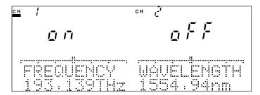
Fig. 4-37 Optical Output ON/OFF Screen
