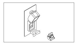
3) Wipe the stain on the end face of ferrule with the adapter cleaner.
