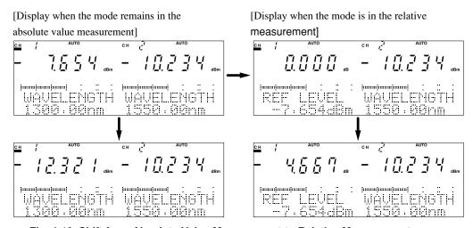
Fig. 4-19 Shift from Absolute Value Measurement to Relative Measurement
