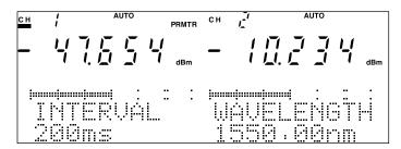
Fig. 4-14 Interval (Fixed Value) Setting Screen
