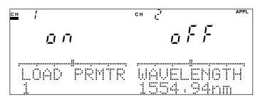
Fig. 4-46 Measurement Condition Reading Screen
