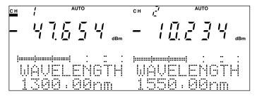
Fig. 4-8 Preset Calibrated Wavelength Setting Screen
