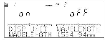
Fig. 4-48 Wavelength Display Setting Screen
