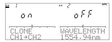
Fig. 4-44 Clone Function Screen
