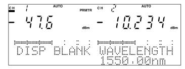
Fig. 4-18 Display Resolution (Blank) Setting Screen
