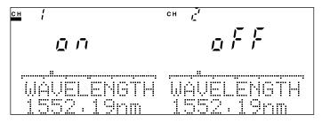
Fig. 4-39 Output Wavelength Setting Screen
