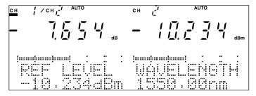
Fig. 4-23 Reference Measurement Screen
