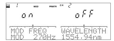
Fig. 4-41 Modulation Mode ON Screen
