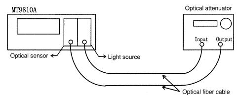
Fig. 4-1 MT9810A Connection Diagram
