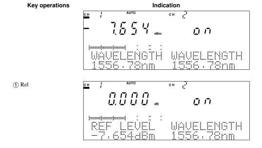
Change the magnitude of attenuation of the optical attenuator in this status. The same value as that of the magnitude of attenuation changed will be indicated.
